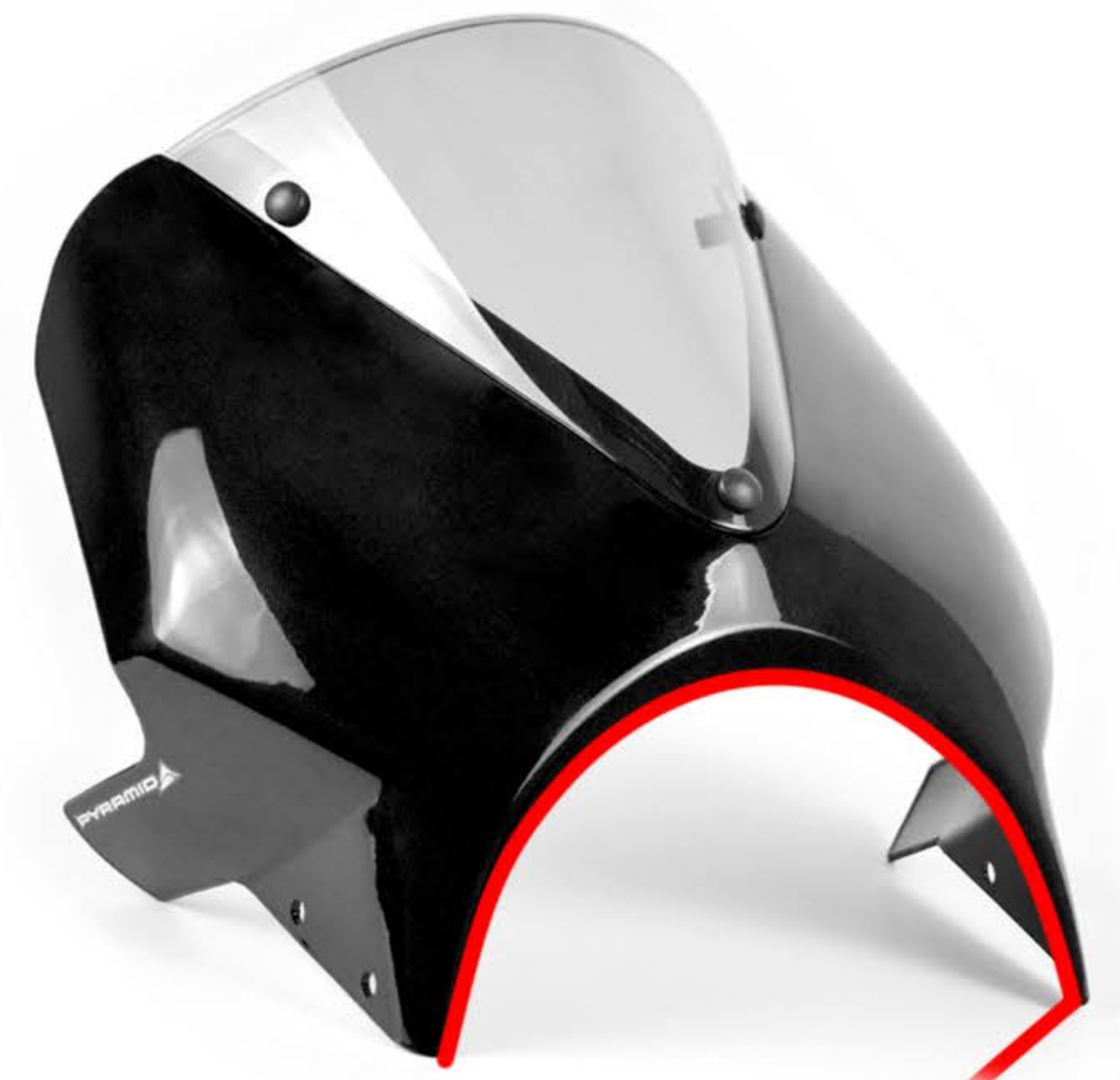
Rubber trim fitted around edge
