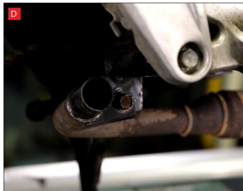
F) Remove the header pipe. You may find that the header studs are corroded, if they are we recommend cleaning these up with a wire brush or if you have one, a die tool.
