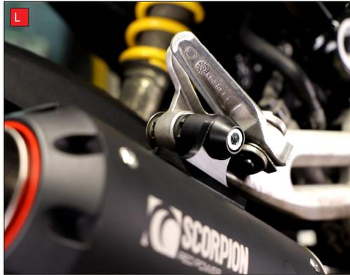
L) Slide the silencer/connecting pipe onto the new header pipe and insert the silencer mounting hardware to loosely hold it in place.
