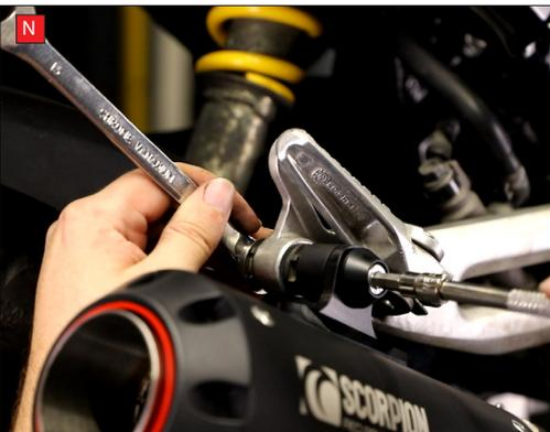
Take the bike for a short ride to ensure it functions as it should. Once the bike and exhaust are cool enough check all nuts and bolts are still secure.
