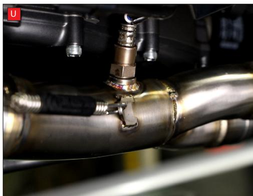
V) Adjust the position of the system to where you're happy that it has clearance around it and there's no stress on any joints, then fully tighten the header nuts, silencer to mounting bracket bolt and mounting bracket to frame bolt.
