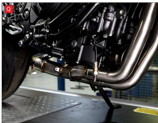
Q) Slide the collector pipe onto the header pipes. The Lambda sensor boss should be on the top.
