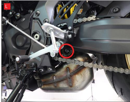
O) Install the new silencer bracket with the supplied hardware as per the diagram.
