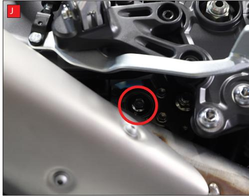
I) Remove the 4 nuts holding the headers to the engine.
