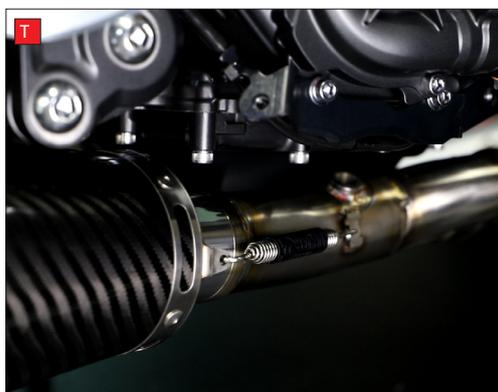
U) Reinstall the Lambda sensor. Before screwing into the pipe twist the sensor in reverse direction several times. This will prevent the cable from being twisting up as you screw the sensor in.
