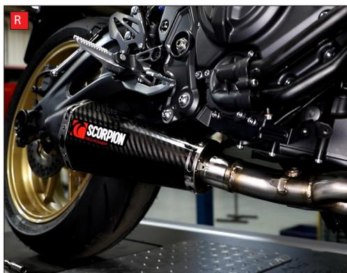
R) Slide the silencer onto the collector pipe. Photo shows the Serket silencer, Red power fits in the same way.
