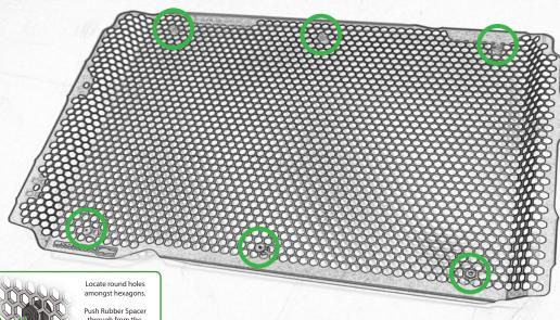
Push Rubber Spacer through from the back of the guard so Hexagonal shape sits on the front face
