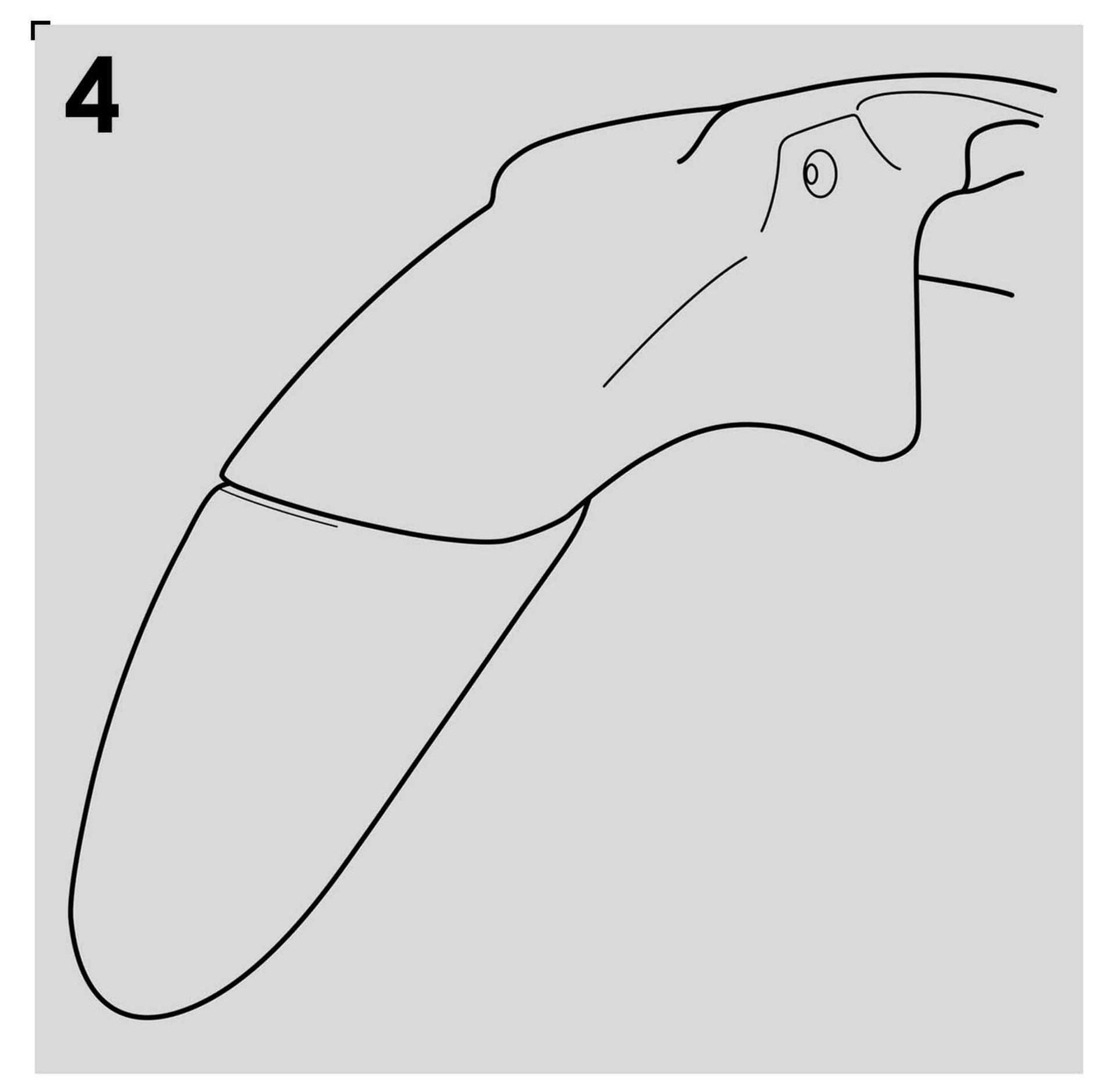
Fit Extenda Fenda/Hugger Extension to mudguard and check for alignment before step 5.
