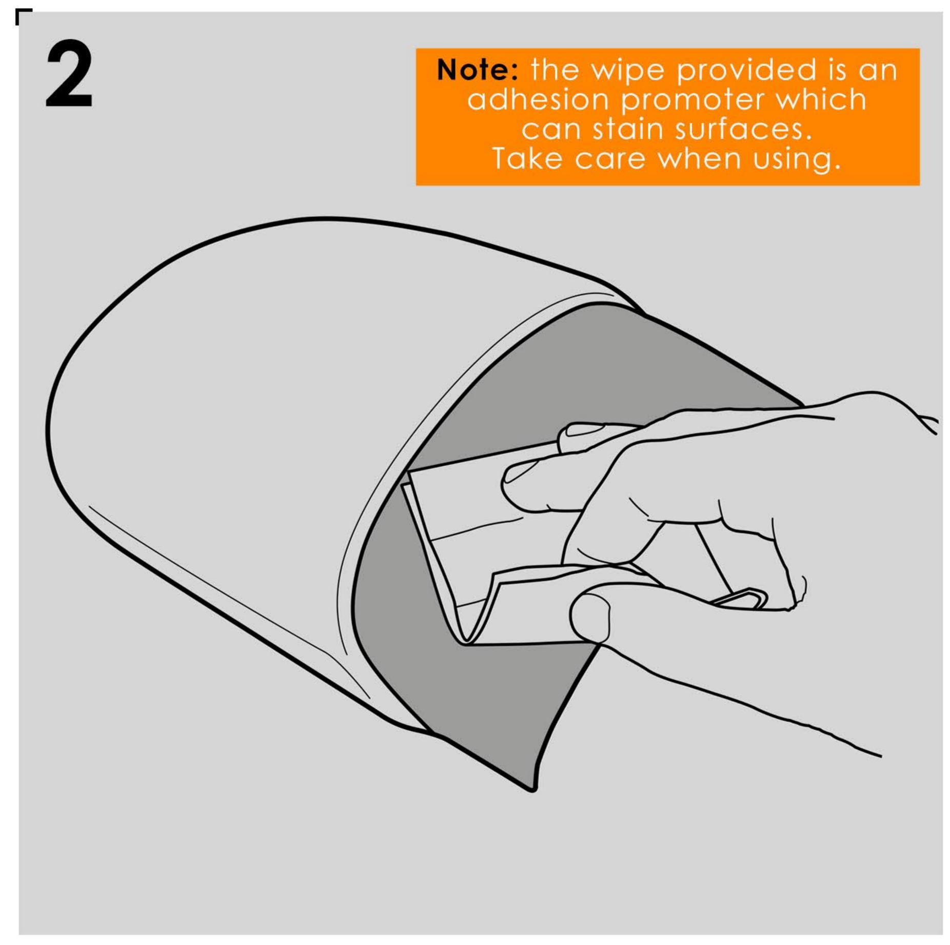
Prime the fitting areas of the OEM mudguard and Pyramid mudguard extension using the wipe supplied.
