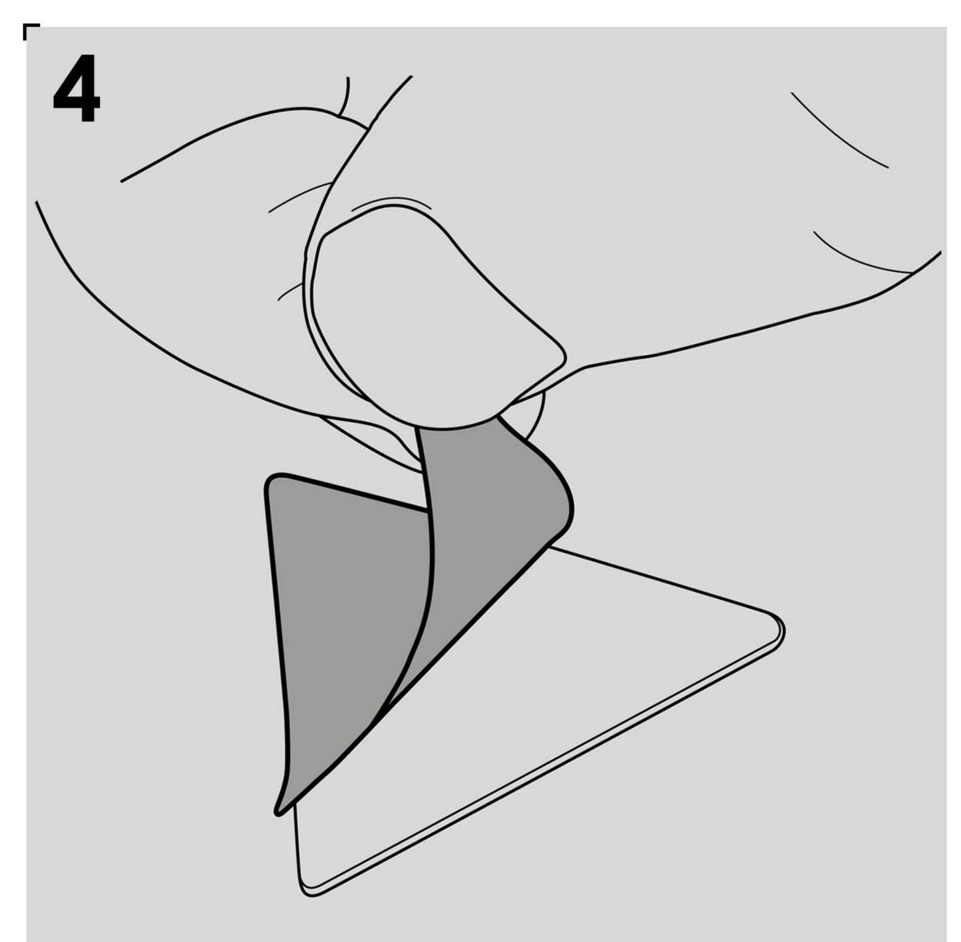
Peel backing paper from Stick-Fit pads.
