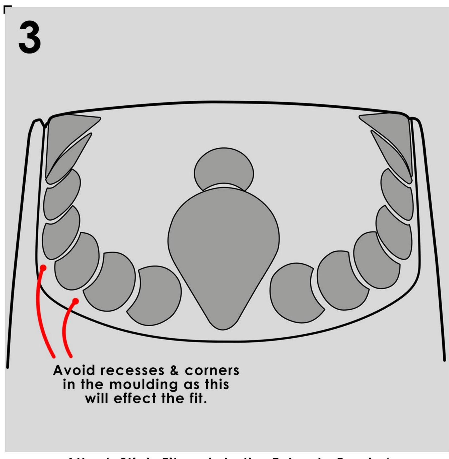
Attach Stick-Fit pads to the Extenda Fenda/ Hugger Extension using this diagram as a guide. Check alignment before step 4.
