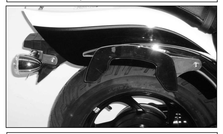
Of course, the assembly requires a certain technical experience. If you are not sure how to execute a determined action, you should ask your local distributor to do it. First, tighten all screws only loosely. After mounting all parts, the screws should be tightened to the torque specified. This guarantees, that the product is mounted without tension. Observe the tightening torques of the manufacturer! Control all screw connections after the assembling for tightness!
