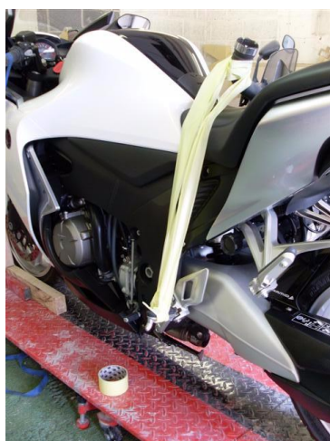
Exhaust strapped to left peg.
