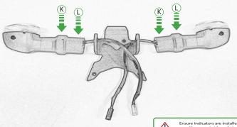
Ensure indicators are installed on the correct sides - drain holes should face down
